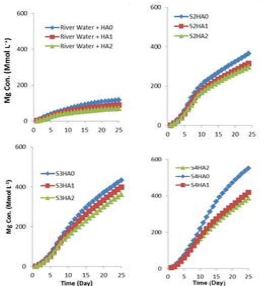
**Figure 3. The relationship between  $\text{Mg}^{++}$  released from water at different salinity levels mixed with different levels of humic acid with time (day).**
