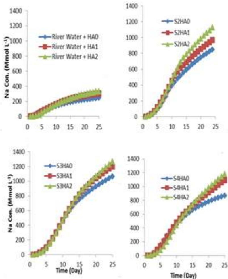
**Figure 1. The relationship between Na<sup>+</sup> released from water at different salinity levels mixed with different levels of humic acid with time (day).**
