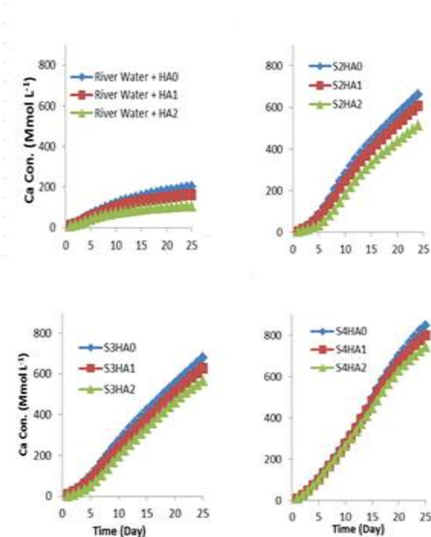
**Figure 2. The relationship between  $\text{Ca}^{++}$  released from water at different salinity levels mixed with different levels of hmic acid with time (day)**
