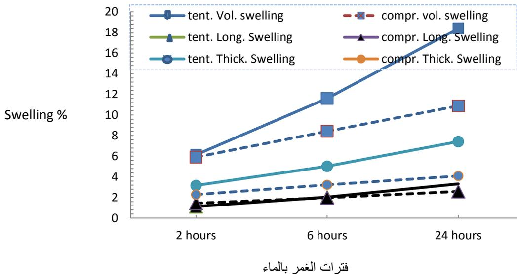
**Figure 6. Differences between tension wood and compression wood in volumetric, longitudinal and thickness swelling percent after immersion in water for 2, 6, 4 hours**
