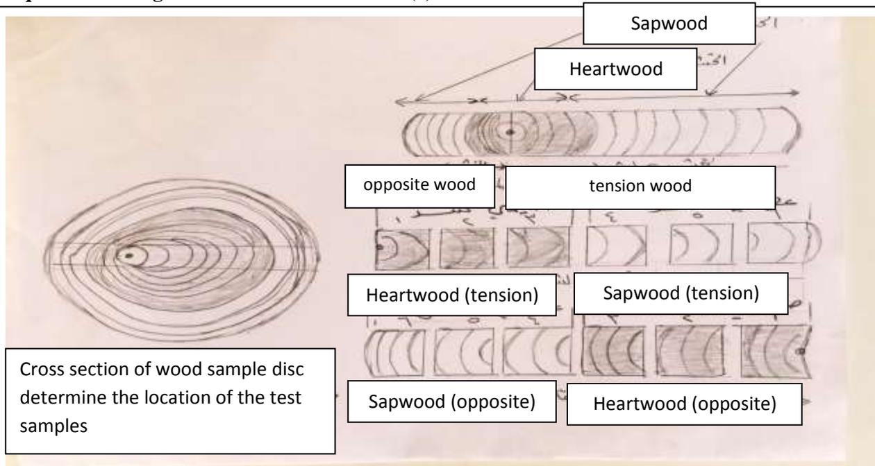
**Figure 2. Physical samples test preparation (for both tension and compression wood)**
