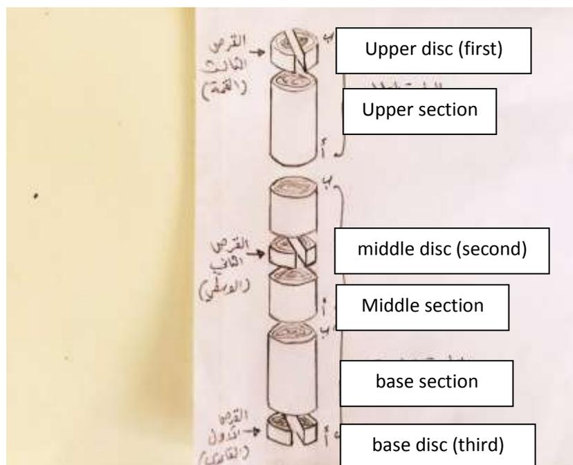
Figure 1. Three stem sections and disc sample preparation used for laboratory tests
