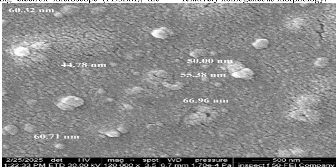
Figure 9. Field Emission Scanning Electron Microscopy image of C/RL-NPs.
